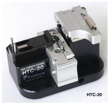
The HTC-20 is designed for cleaving single count of silica optical fiber by keeping the cleaved fiber's glass surface free from any physical contact. (The glass portion of the fiber is not on the fiber pad.)
