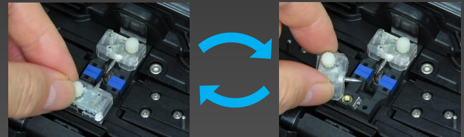
Electrode replacement without tools
