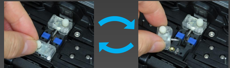
Electrode replacement without tools
